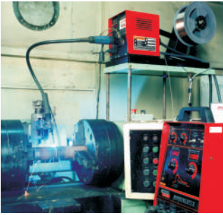
Fully automated tube to tube TIG Welding Machine
